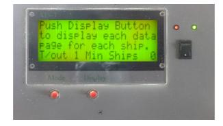
'Monitor Ship': The cursor cycles through the ship numbers, from 0-9, upon pressing the Display button. After 9, the cursor goes back to the Reset menu item at the top of the screen. When you have the desired ship number, press Mode and the SRS-1 will monitor that ship, much like the monitoring of the closest ship. Reset using the Reset option.
